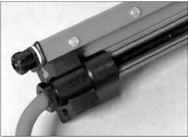
Fig. 6: HAUG ionizing bar, combined with air-assisted "Jet Streamer" for the removal of dust from surfaces and for the transport of generated ions to greater distance.
