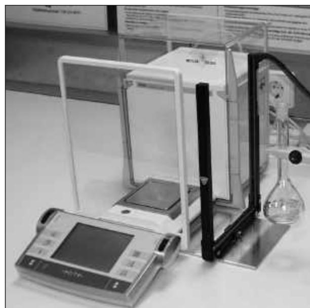
ill. 2: An ionizer in front of the weighing area of an analytical scale ensures that weighed materials are electrically neutral.
